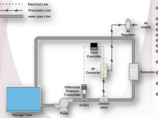
The controller can be connected to computer through comport for monitoring the process in SCADA.
